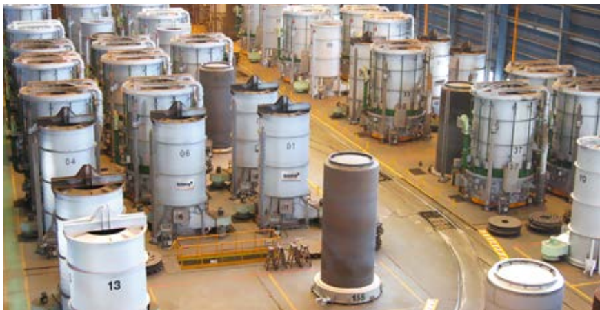
▲ HPH® Bell-type Annealing Plant for cold-rolled steel strip, equipped with 99 bases
