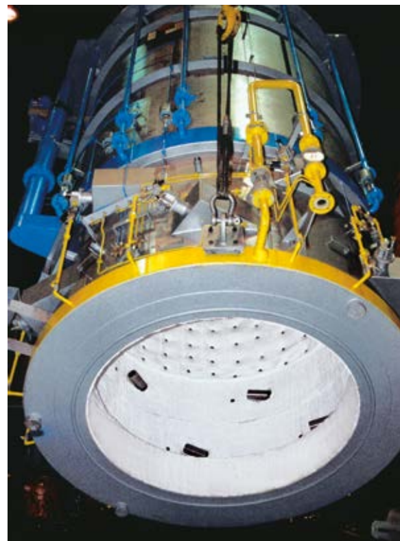
▲ Heating hood of an HPH® plant – special fibre insulation for very low heat losses and low NO x burner technology
