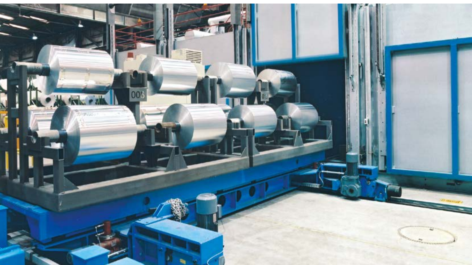
▲ Multi-chamber annealing furnace ▼ for annealing of foil coils FAL.
